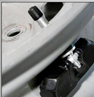
Valve options for 0.453", 0.625", and 7.7mm rim holes
