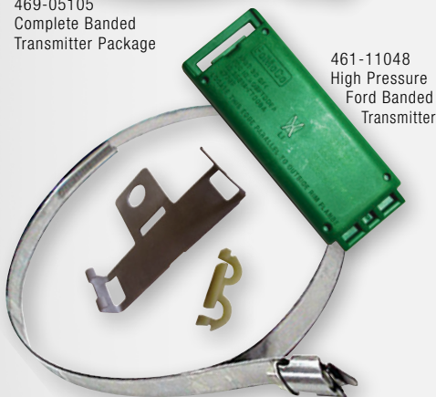
469-15105 Ford Complete Banded High Pressure Sensor Package
